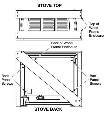
Figure 4 - Unpacking Stove from Wooden Shipping Enclosure
